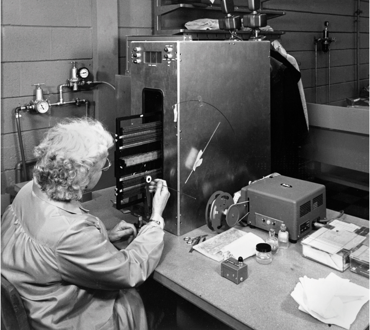
6 A factory worker at Raytheon in Waltham, Massachusetts, hand-weaving a “rope core” memory unit for the Apollo computer. Using this painstaking technique, it took six weeks to manufacture the software for a single Apollo computer.
